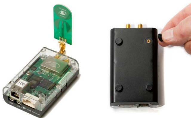
Fig. 4-25: P440 in standard enclosure (left) and view of enclosure bottom showing feet and mounting holes for 4-40 screw
