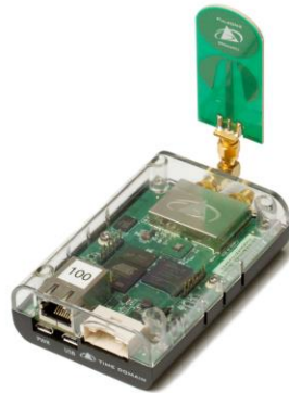
Fig. 1: P440 UWB Module with attached Broadspec Antenna
